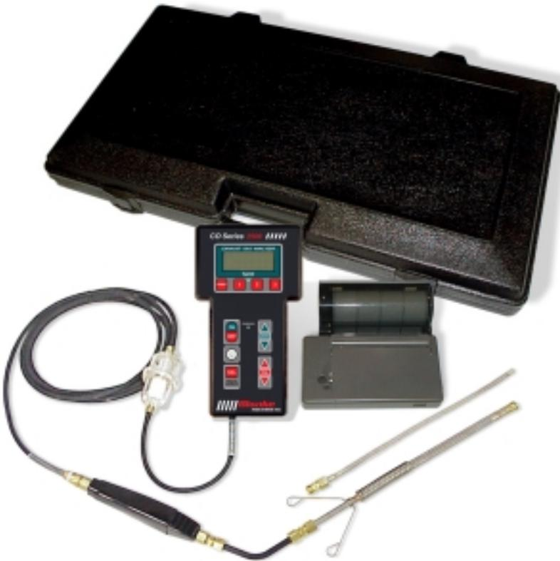
Monitoring exhaust emissions is not only important to help control pollutants, it also helps maintain optimum fuel efficiency and extend engine life. This tool will let the operator quickly determine the general health of an engine. With the CO Series 2500, any engine can be properly tested and repaired to assure ideal engine performance.
